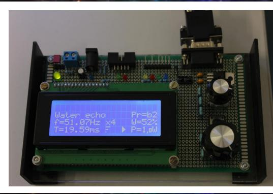
Depending on frequency of the pulses the light of the stroboscope can create various images. The controller we constructed generates frequencies in the range from 1 - 800 Hz.
